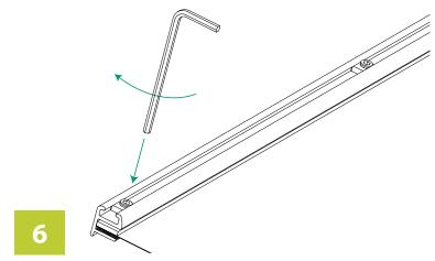
Tighten up grub screws to secure graphic.
