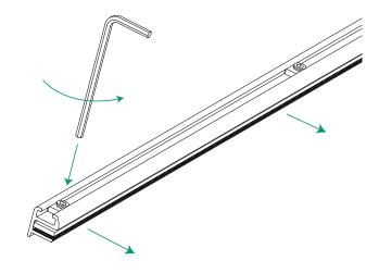
Undo grub screws and remove graphic guide.
