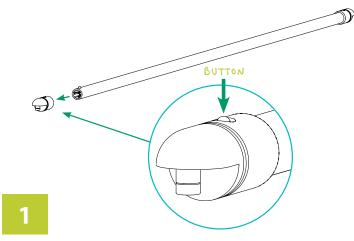
Press button to remove cross arm ends.
