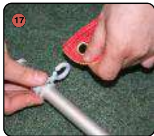
Take the bottom horizontal edge of the graphic and attach each eyelet onto the plastic hooks on the bottom bungee pole. Space out evenly. For double sided display repeat steps 14 to 17 for the 2nd graphic
