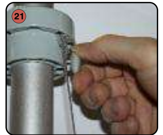
Lock the telescopic support pole into place. Repeat for the 2nd support pole.
