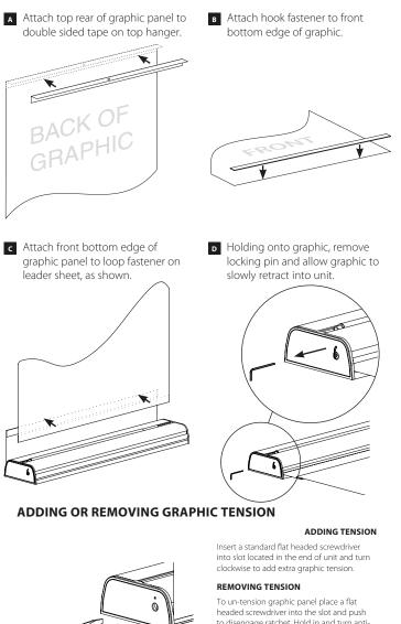
to disengage ratchet. Hold in and turn anticlockwise until tension in spring is released. To remove graphic panel carefully peel it off leader sheet. The graphic hanger can also be removed or a new hanger can be purchased.
